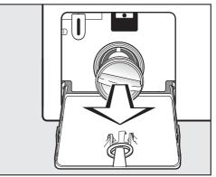
■ Remove the drain filter completely.
